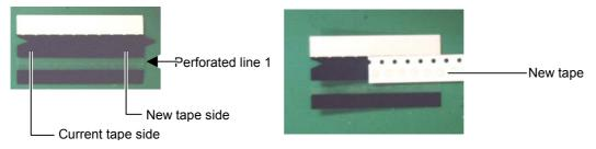
Step 3 Attach the current component tape on the left half of the joint tape with its cover tape side facing the joint tape, its sprocket-side edge aligned to the plastic guide.
