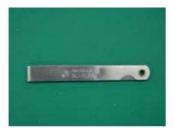
■ Spring scale(KJ3-MJ154-00, BAR TYPE TENSION GA.)
